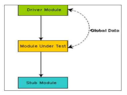
Unit testing with the help of driver and stub modules
